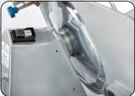
Switches mounted on top to reduce failures
