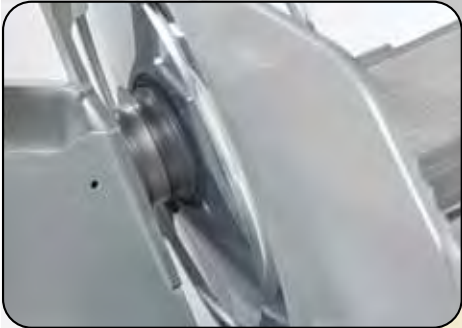
Wide gap between blade and housing for more thorough cleaning
